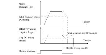
Figure 5-9:Schematic diagram of stop DC braking time
