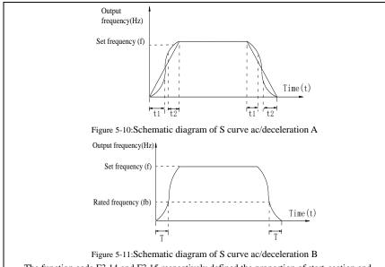
The function code F3.14 and F3.15 respectively defined the proportion of start-section and the proportion of end-section for S curve acceleration and deceleration A, the two function code must meet:  $F3.14 + F3.15 \le 100.0\%$ .
