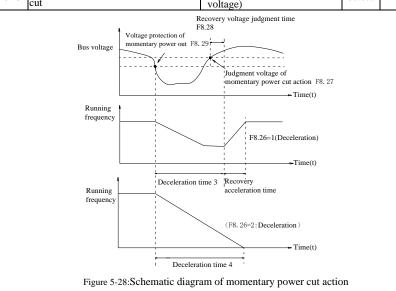
This feature means that when the momentary power cut happens or the voltage suddenly reduces, the drive will reduce the output speed to compensate the reduced value of the inverter DC bus voltage by using load feedback energy, in order to maintain the inverter to continue running.
