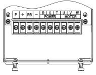
Figure 4-6: 15kW G3 main circuit terminal
