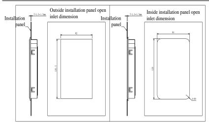
Figure 7-13:ST500 keyboard installation open inlet dimension(mm)
