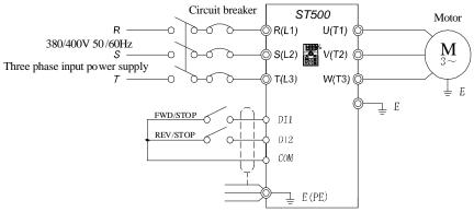
Terminal control of positive and reverse motor
