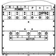
Figure 4-12: 160kW~220kW G3 main circuit terminal
