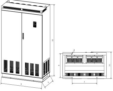
Figure 7-9: 450kW~630kW G3 (DC reactor) dimension **Iron shell standing installation series**
