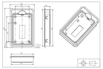
Figure 7-12:ST500 Keyboard dimension (mm)
