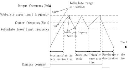
Figure 5-29:Schematic diagram of wobbulate operating
