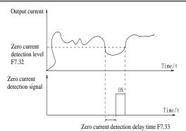
Figure 5-25:Schematic diagram of zero current detection
