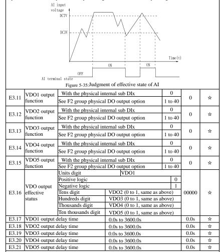
VDO and DO output function is similar, can be used in conjunction with VDIx, to achieve some simple logic control.
