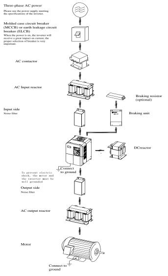
Figure 9-1: Wiring of optional accessaries.
