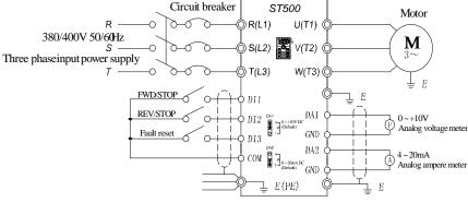
External frequency meter and ammeter
