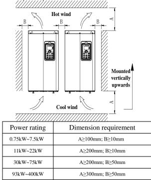
Figure 4-1: ST500 Series Each power level installation space requirement
