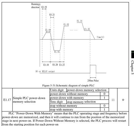
PLC "Stop With Memory" means that the PLC operating stage and frequency before stop are recorded, and then it will continue to run from the position of the recorded stage in next run. If Stop Without Memory is selected, the PLC process will restart from the starting position for each start.
