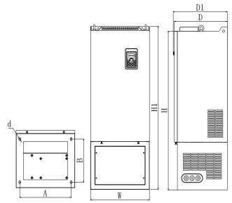
Figure 7-6: 132kW G3 (Base with DC reactor) Outline dimension
