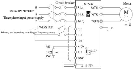
Frequency given mode (external potentiometer, keyboard encoder) switching
