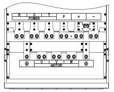
Figure 4-13: 250kW~400kW G3 main circuit terminal 11.450kW~630kW G3 main circuit terminal
