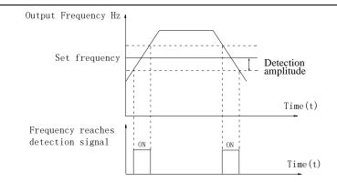
Figure 5-23:Schematic diagram of frequency arrival detection amplitude
