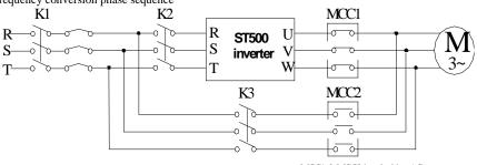
MCC1 & MCC2 interlocking AC contactor
