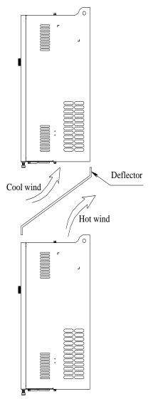
Figure 4-2: Heat insulation deflector up and down installation diagram
