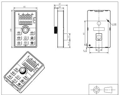
Figure 7-11:ST500 Keyboard dimension (mm)
