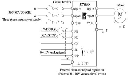
**V-9-2 Connection:** The (+) terminal of the external analog signal is connected to the AI1 terminal, and the other terminal of the signal is connected to the GND terminal of the inverter.
